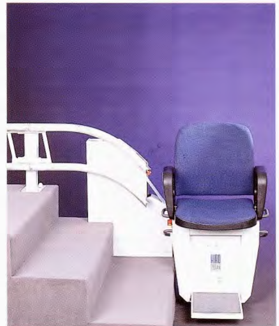
The folding track (Extras) is used for situations where a door is present and may not be blocked. In the neutral position, the track ends flush with the first step. For the downward ride, the track is lowered, complete with passenger for easy access. For the upwards trip, the track is folded back automatically into its normal position, thus leaving the corridor clear.
